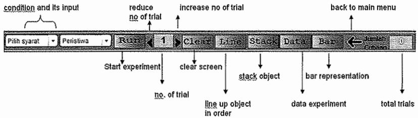
**Figure 4 Identical Layout in Each Microworld of the WPE**
