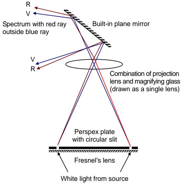
**Figure 4b: Circular Spectrum Projected on a Screen With a Rainbow Color Sequence**
