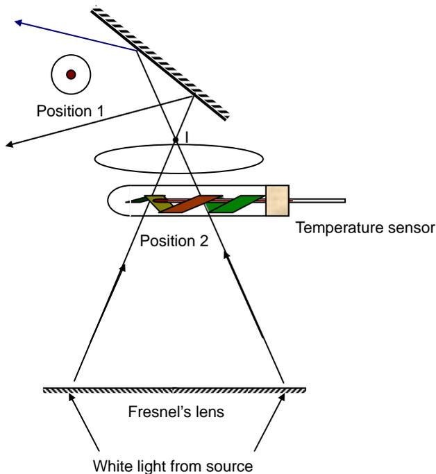
For safety, the level of projection lens should be adjusted before the experiment so that the image of the filament is formed just above the projection lens, and the boiling tube should be placed 10 to 15 cm either below the image (Position 1) or the same distance in front of the image (Position 2). In these positions, the light intensity will create a rise in temperature at a rate of 2–5 °C per minute, but not too strong to overheat the temperature sensor.
