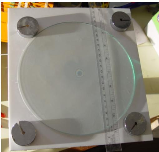
Note: Light comes from an OHP on the left with an incident angle about  $85^\circ$ . The central slotted weight is under the Perspex plate where Newton's rings are seen.
