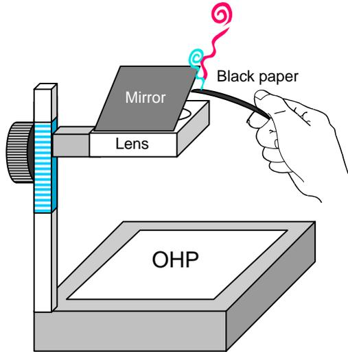
Under normal circumstances, smoking will not damage the projection system because both the lens and the mirror in this part are made of heat resistant glass. However, the soot left on glass surfaces is difficult to clean if unattended for some time. The stain should be removed immediately with diluted alcohol after the demonstration.
