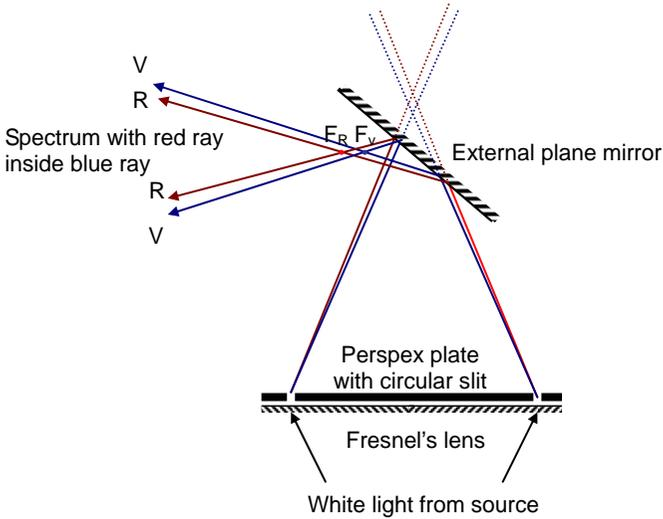
**Figure 3b: Circular Spectrum Projected on a Screen With a Reversed Color Sequence**
